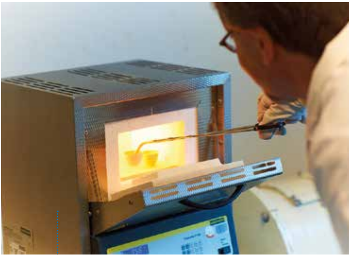
To complete the chemical analysis, the quicklime is heated in a furnace in two steps, first to 550°C and then to 1025°C.
