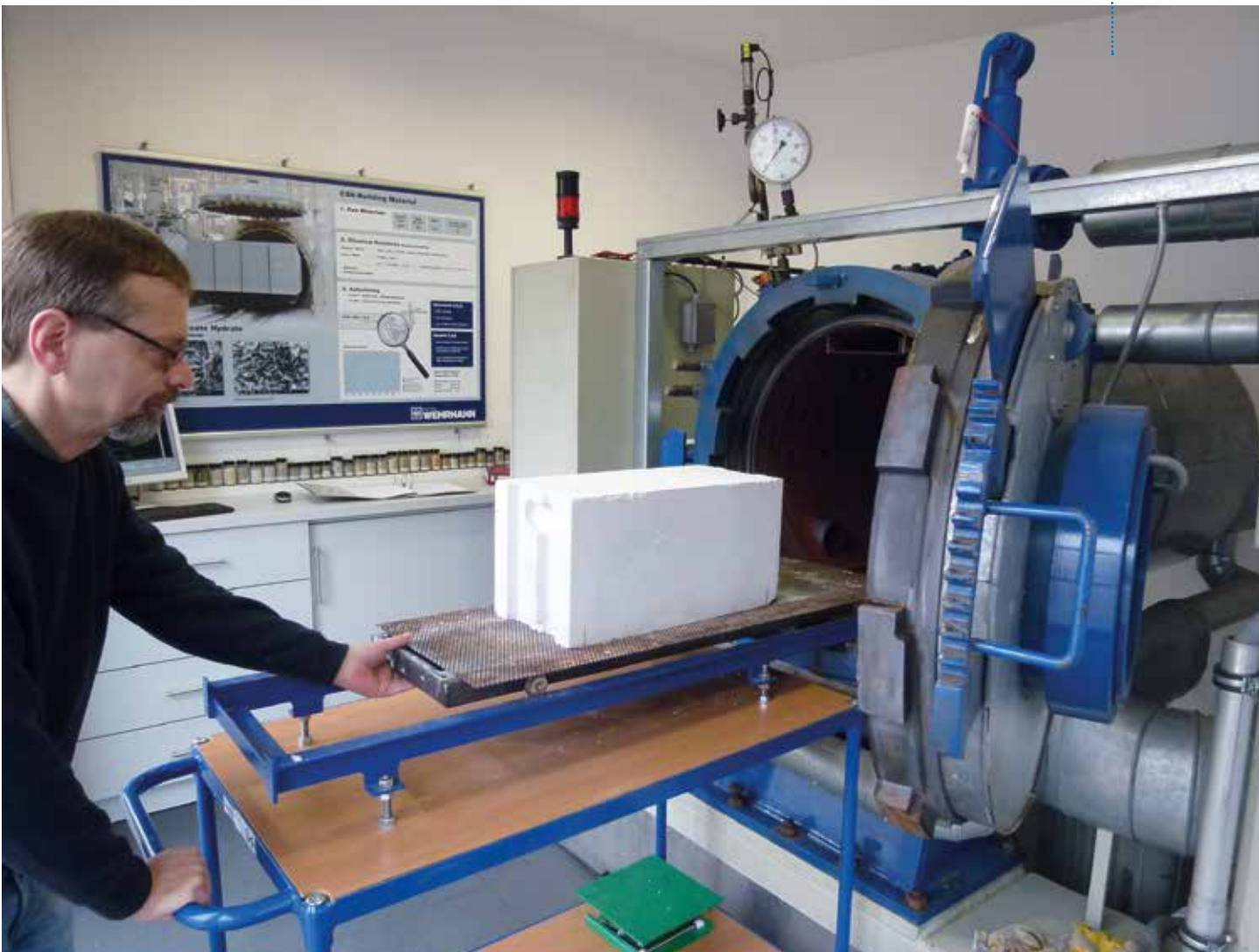
During the precuring process, the temperature and the rising of the green cake is continuously monitored until a sufficient hardness and cake height is reached. Afterwards, the green cake is autoclaved in the Wehrhahn laboratory autoclave with a volume of 500 l.
