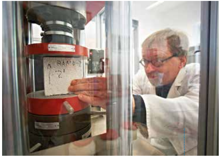
The compressive strength is determined at cubes of 100x100x100 mm using an electronically controlled testing machine according to DIN EN 772-1:2011-07.
