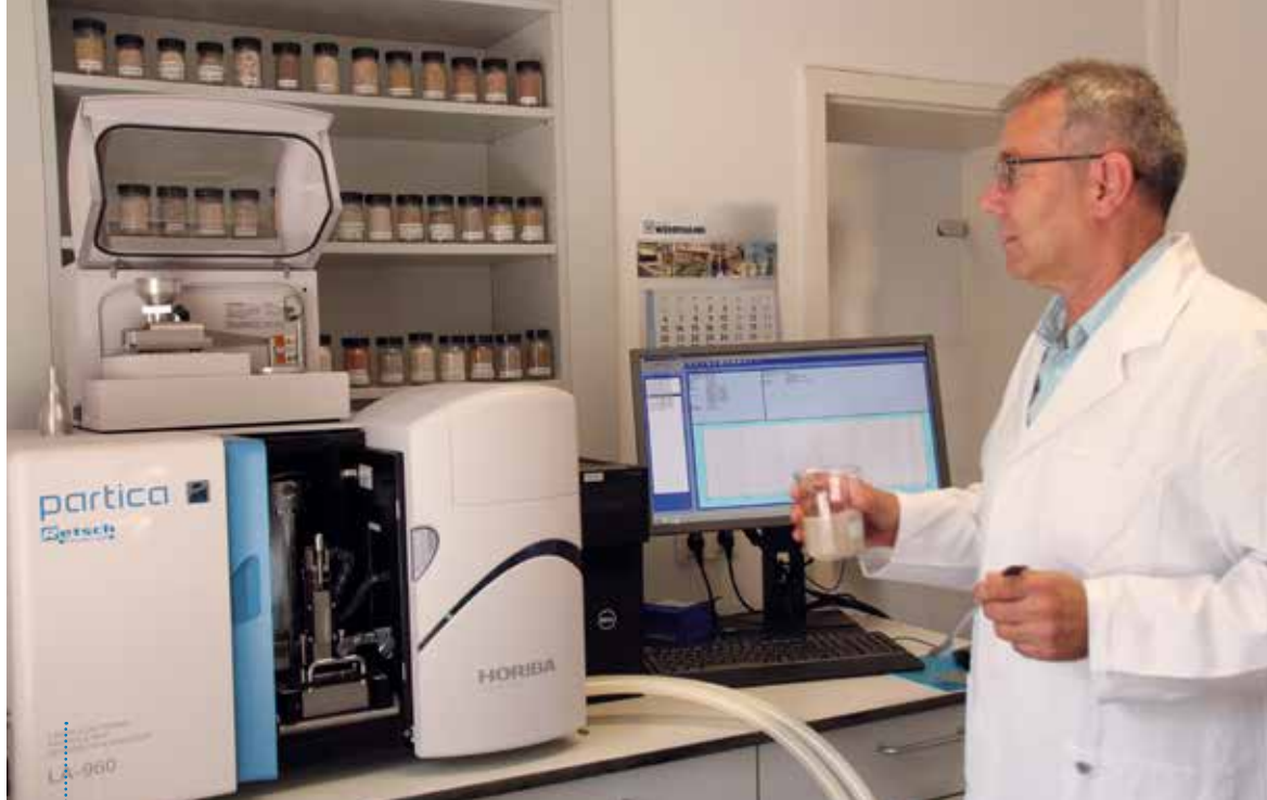
A laser scattering particle size distribution analyser even detects particles down to 0.1 µm in detail, whereas traditional sieving methods with air jet sieving or vibration screening machines are limited to 32 µm.
